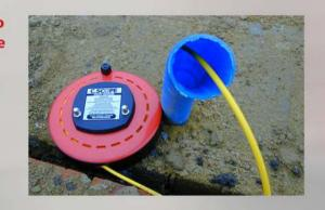
Use a transmitting Sonde to propel along a pipe - tracking its progress using the C.Scope **Cable Avoidance Tool**
